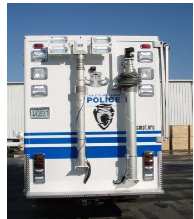
NightVision camera on a 34-ft pneumatic tower and multi-directional 20-ft light tower.
