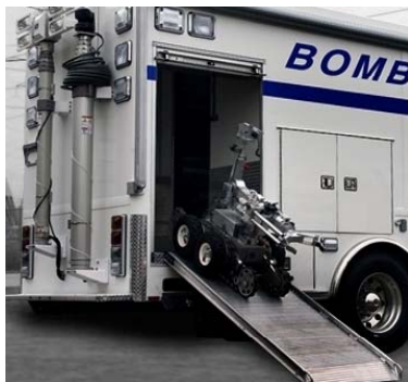
Robot is rapidly deployed from the garage by a ramp that stores beneath the floor.
