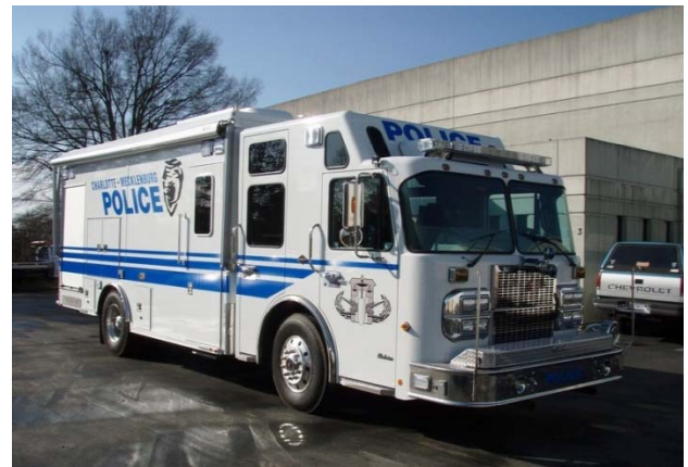
Front bumper compartments provide storage for rapid deployment of forcible entry tools.
