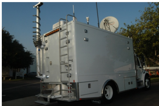
A 25-ft tower with surveillance camera, rapid deploy antenna, including cellular transceivers and AVL SAT dish. A rear mounted ladder provides safe access to a anti-slip tread plate roof. Fold-down steps provides safe entrance and exit to the interior.
