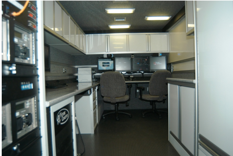
Two primary work stations are on the forward wall with one auxiliary work station on the street side wall. The four 20" LCD monitors at the forward work station are all linked allowing any individual view to be dragged from monitor to monitor, acting virtually as a single panoramic monitor.
