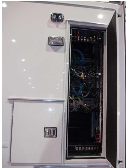
All electronics are easily accessed for service through the two exterior compartment doors. The lower compartment door(not shown) beneath the doors folds down to provide a work platform. Doors are heavily insulated and soundproofed.
