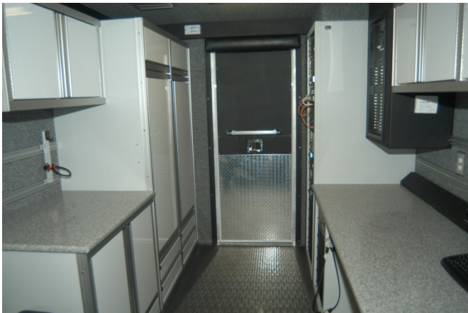
Looking back toward the rear door. Additional equipment mounting rails are provided along the full length of both walls allowing mounting of additional monitors and other equipment. Note the back wiring traces at the back of the work stations permitting simple routing of cables from the electronics cabinet to any work location as the vehicle is upgraded at a future date.
